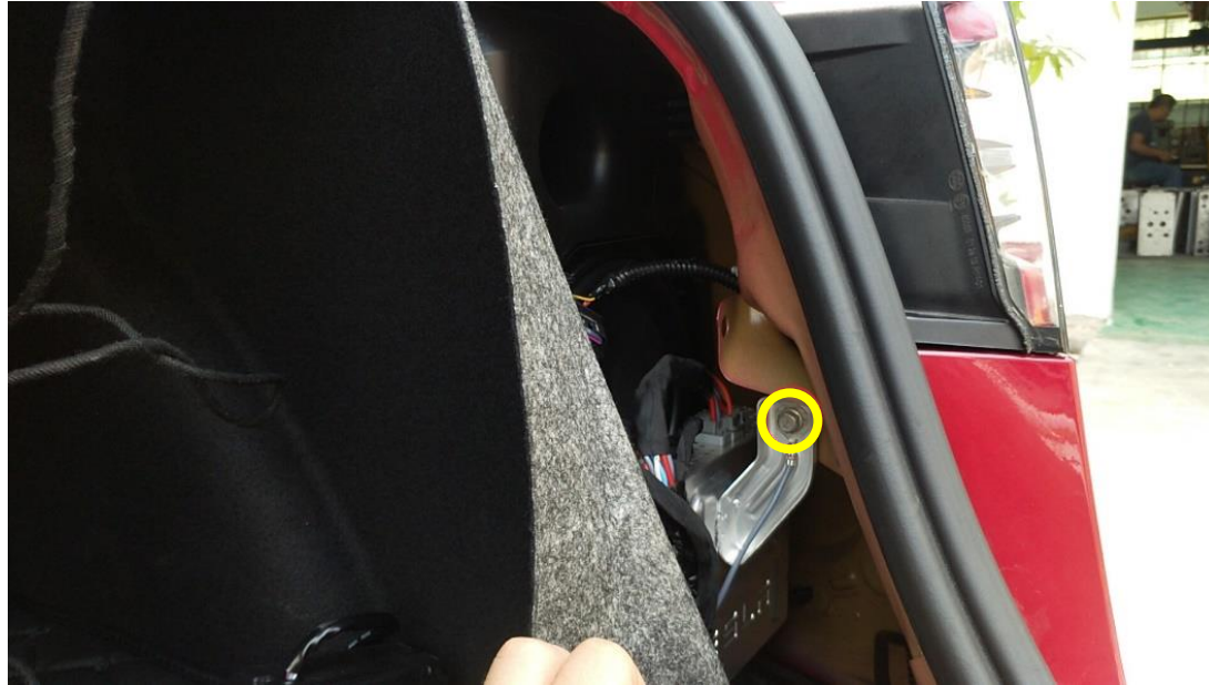
Figure 1 (Ground inside the trunk)
