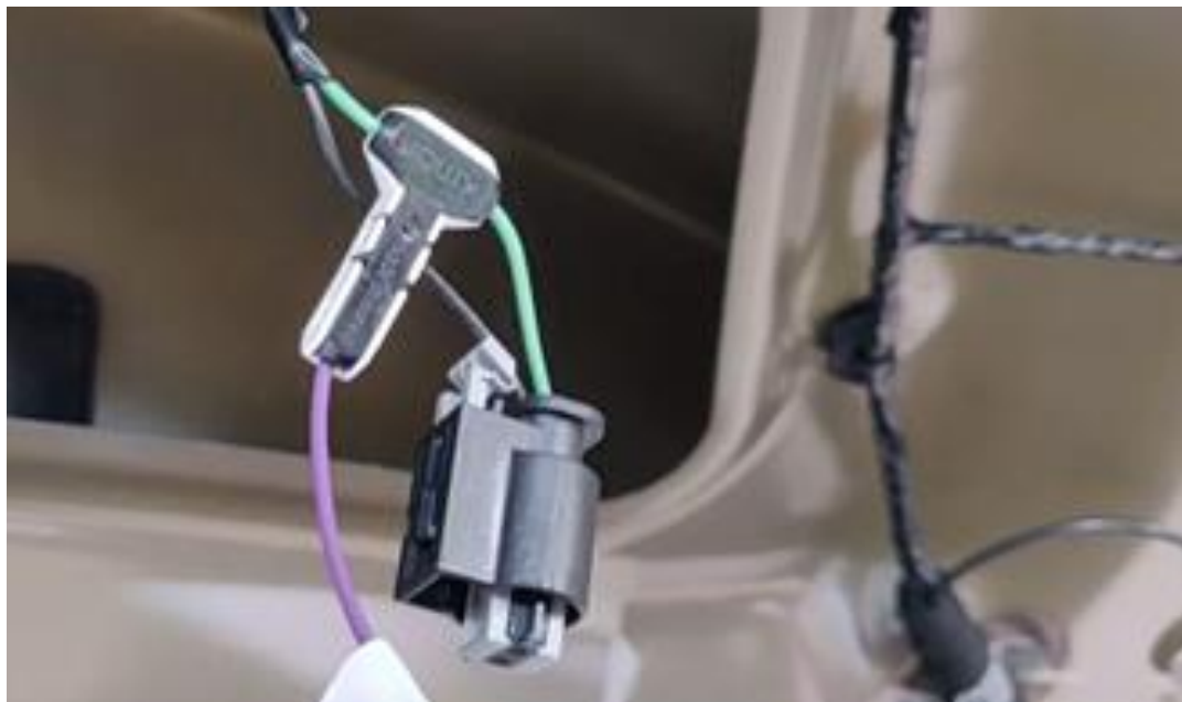
Figure 5 (Tap the purple wire into the green wire*)
