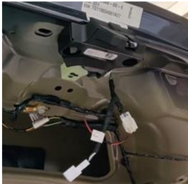
Figure 4 (Use the Y-connector to connect to the lock control)
